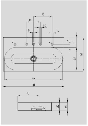
\* Control knob holes for CLOU waste and overflow system with cable operated pop-up waste and deck mounted control knob, optionally left or right
